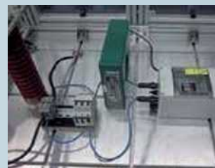
SCB during a surge load test
